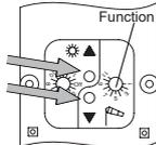
Press the **DOWN** and **UP** buttons **at the same time.** **min. 3 sec.** Transmission LED (flashes briefly)
